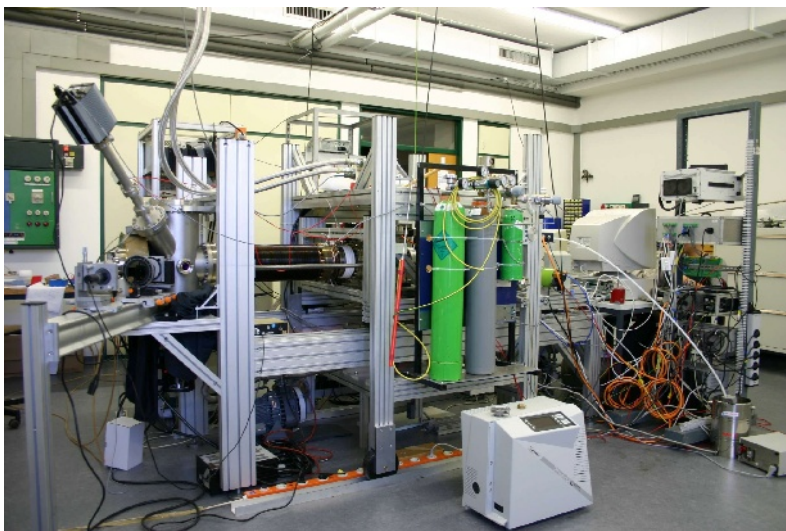
Calibration electron sources, e.g. angular-selective pulsed UV-laser photo-electron source
