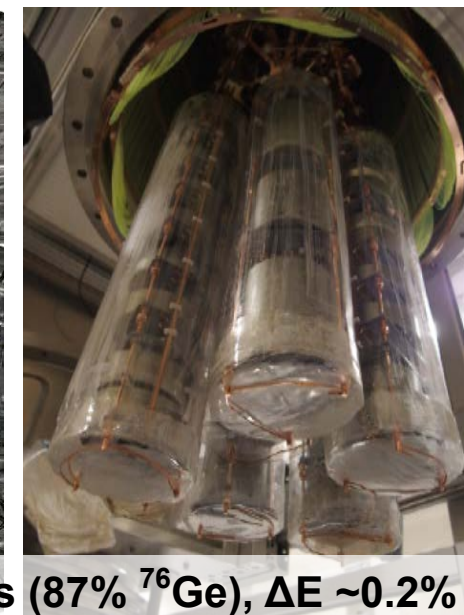
44 kg of Ge crystals (88% ^{76}\text{Ge} ), \Delta E \sim 0.1\%
